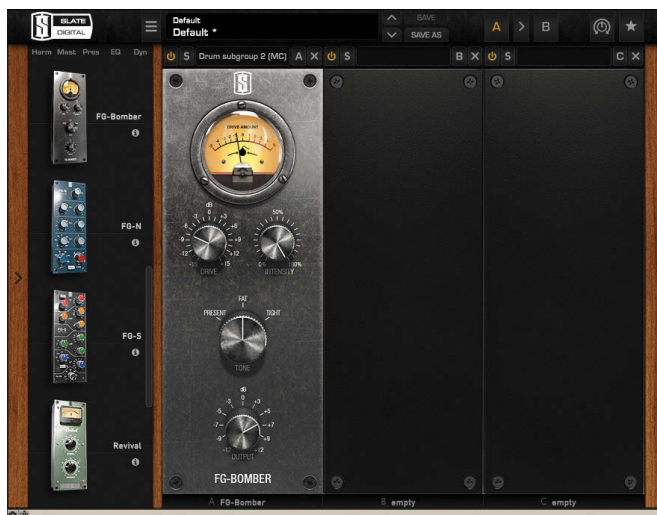
Figure 1: FG-Bomber is loaded here into the first slot of the Virtual Mix Rack plug-in, an expandable rack that can host up to eight compatible Slate Digital modules. Other modules in the browser (located to the left of the rack slots) can be dragged into empty slots.
